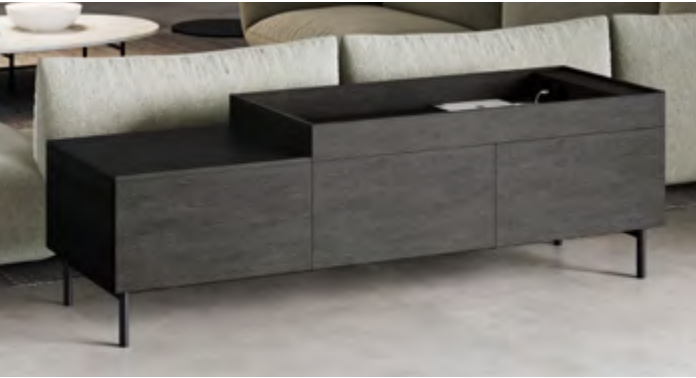
base frame with rod legs 17.5 cm high, ø 2.5 cm in matt lacquer and O20 black Base frame are possible for sideboards up to a height of 4 modules. From a width of 160 cm, a centre leg is required for 3 and 4 module heights. Hinge-door modules can be planned on base frames up to a height of 5 modules. rod feet are indented 4 cm from the outer edges.
